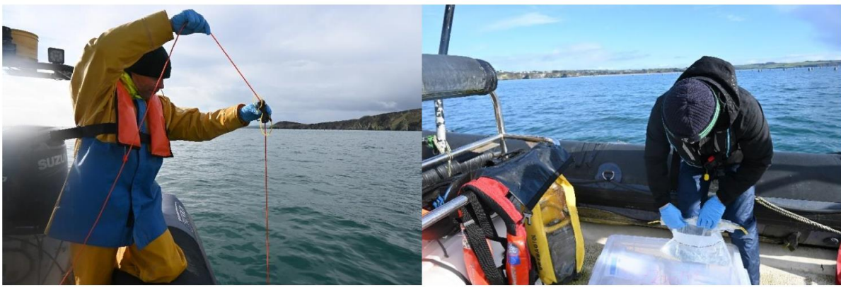
Figure 13 Deploying the Niskin bottle to take water sample at depth (left) packing sample to be taken back for filtering (right).
